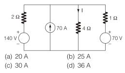
Q.13 For the network shown in the figure below, what is the voltage across the current source?
