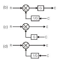
Q.10 The below shown feedback control system has to be reduced to equivalent unity feedback system. Which one of the following is equivalent?
